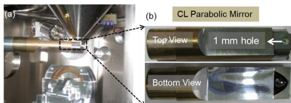
**Figure 3:** (a) Photograph of the CL parabolic mirror and SEM pole piece. (b) Zoomed view of CL parabolic mirror (views from top and bottom).
