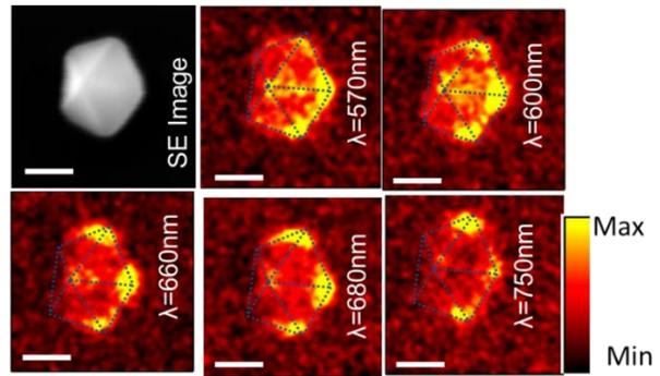
**Figure 5.** Monochromatic CL emission maps on an isolated gold decahedron on silicon.
