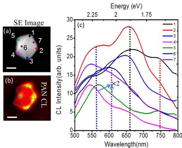
**FIGURE 4.** a) SEM image and (b) corresponding panchromatic CL image on an isolated Au decahedron of side edge length 220 nm. (c) Experimentally obtained CL spectra from different beam injection positions of the decahedron. The SE image shows the e-beam impact points (marked as 1, 2, 3...7) with different colored dots.
