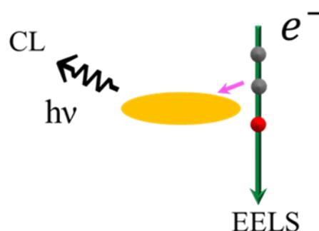
**Figure 1.** Schematic diagram of the basic principle of cathodoluminescence in metallic nanostructures.
