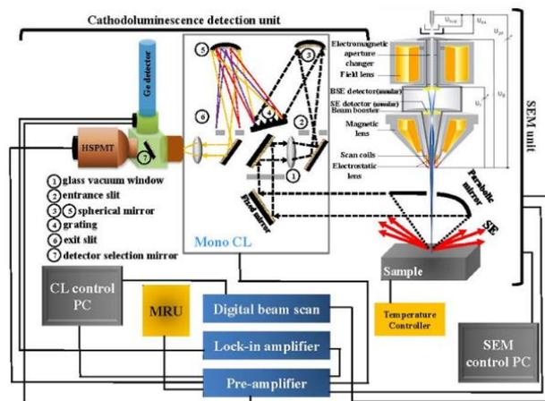
**Figure 2.** Schematic diagram of cathodoluminescence in scanning electron microscope (CL-SEM) system installed at the Saha Institute of Nuclear Physics, Kolkata. Image adapted from Ref. 6.
